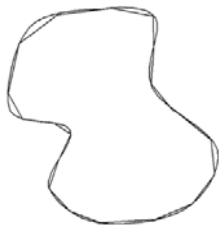
Fig. 2 The boundary represented by a set of straight-line panels [10]
